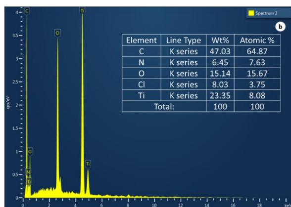
Fig. 7. EDAX spectrum of the TiO<sub>2</sub>-PANI nanocomposite
