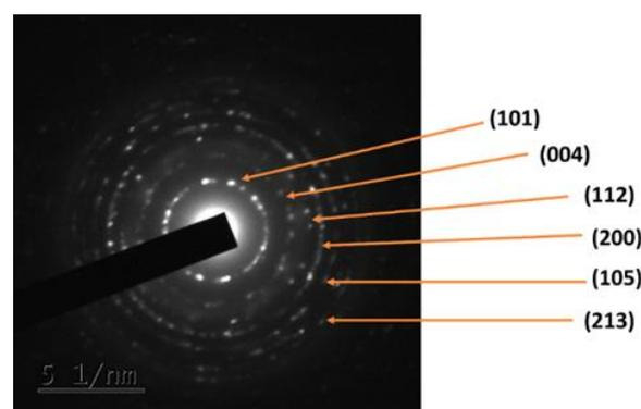
**Fig. 12.** SAED pattern of the TiO<sub>2</sub>-PANI nanocomposite
