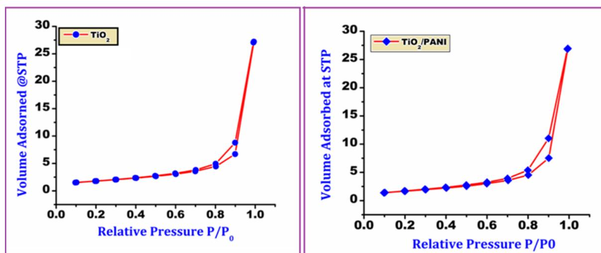
Fig. 13. Brunauer-Emmett-Teller nitrogen adsorption-desorption spectrum for bare TiO<sub>2</sub> and TiO<sub>2</sub>/PANI nanocomposite material
