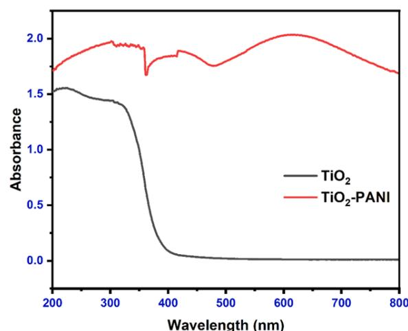
Fig. 1. Absorbance Spectra of the bare TiO<sub>2</sub> and TiO<sub>2</sub>-PANI nanocomposite
