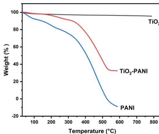
Fig. 9. TGA of PANI, TiO<sub>2</sub>, and TiO<sub>2</sub>-PANI nanocomposite
