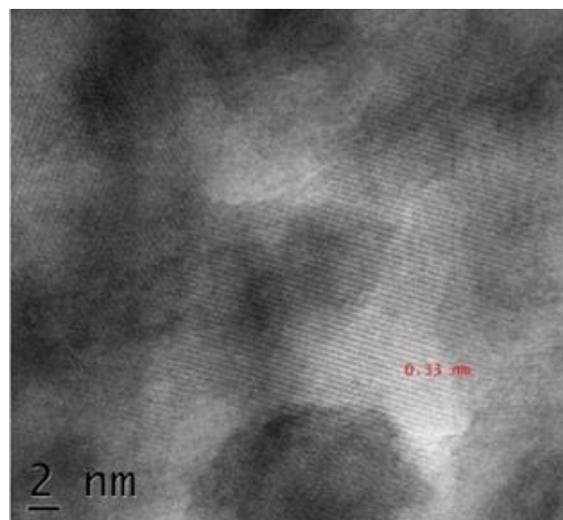
**Fig. 11.** Lattice spacing in TiO<sub>2</sub>-PANI nanocomposite
