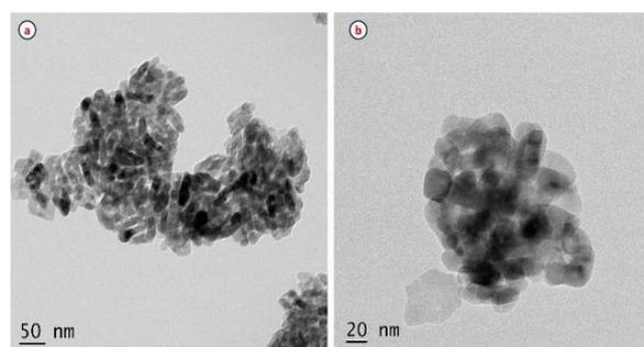
**Fig. 10.** TEM of TiO<sub>2</sub>-PANI nanocomposite
