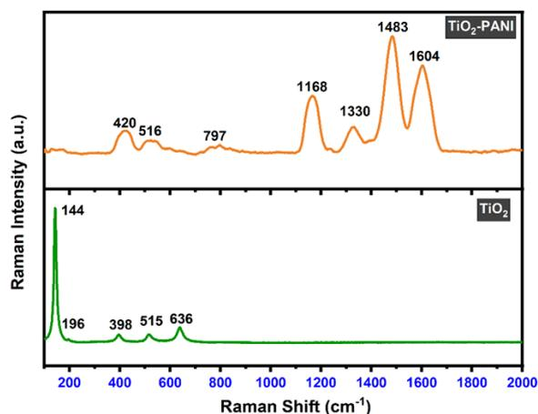
Fig. 8. Raman spectrum of the prepared material
