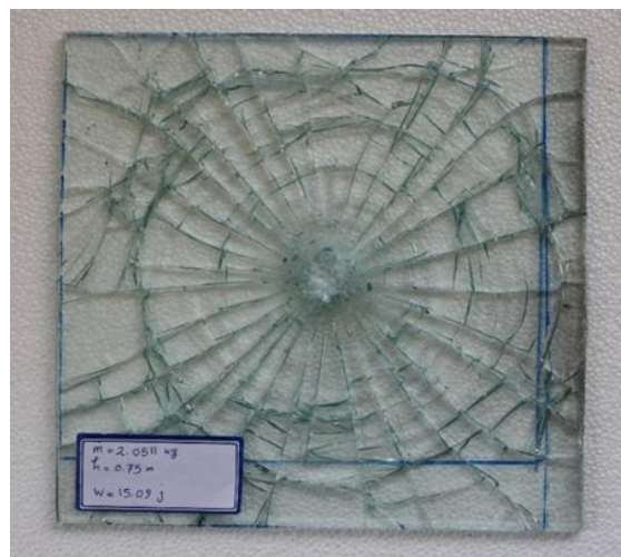
Fig12. .specimen after test code D-B-T-5
